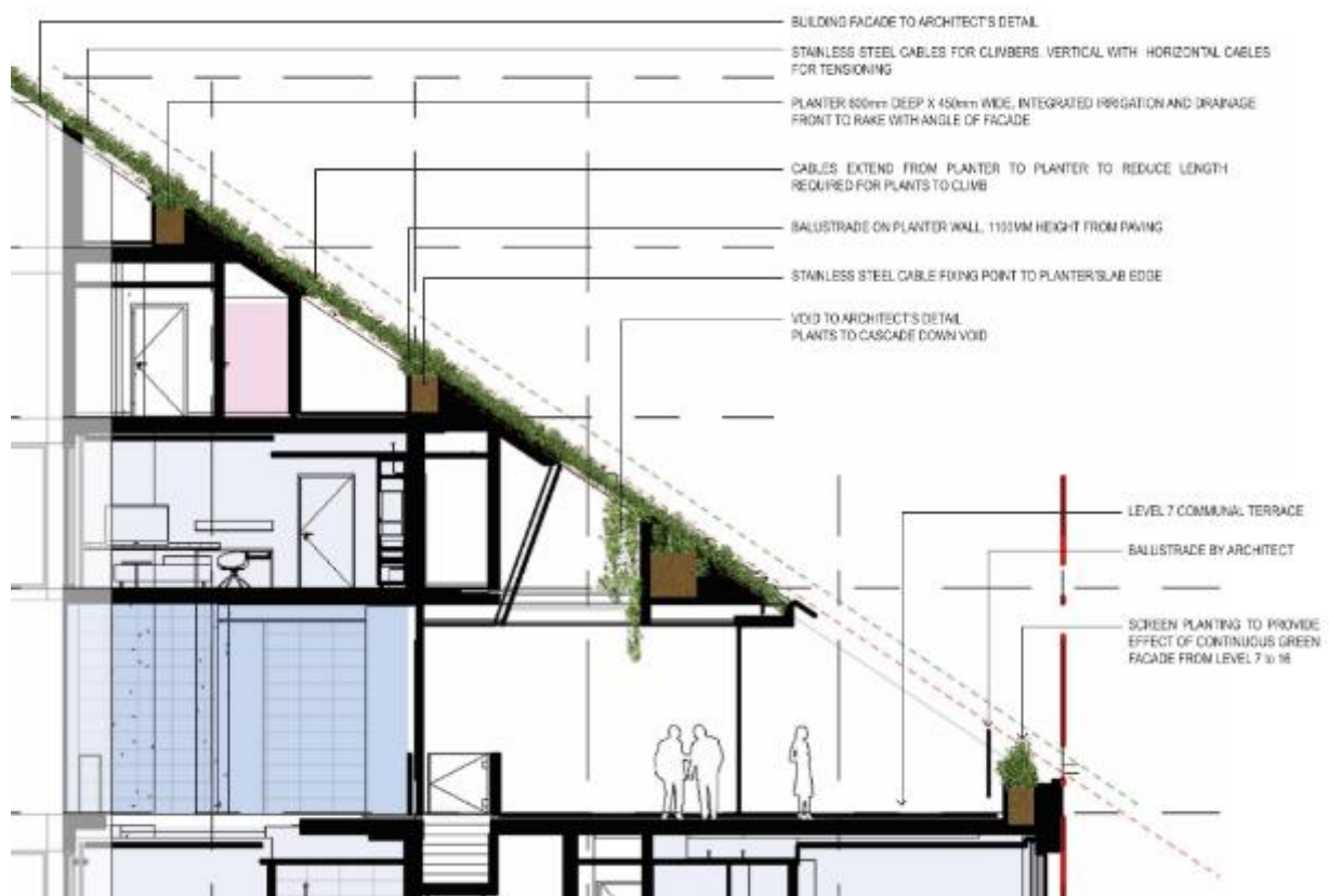
Figure 23: Detailed section of the upper level facade planting
