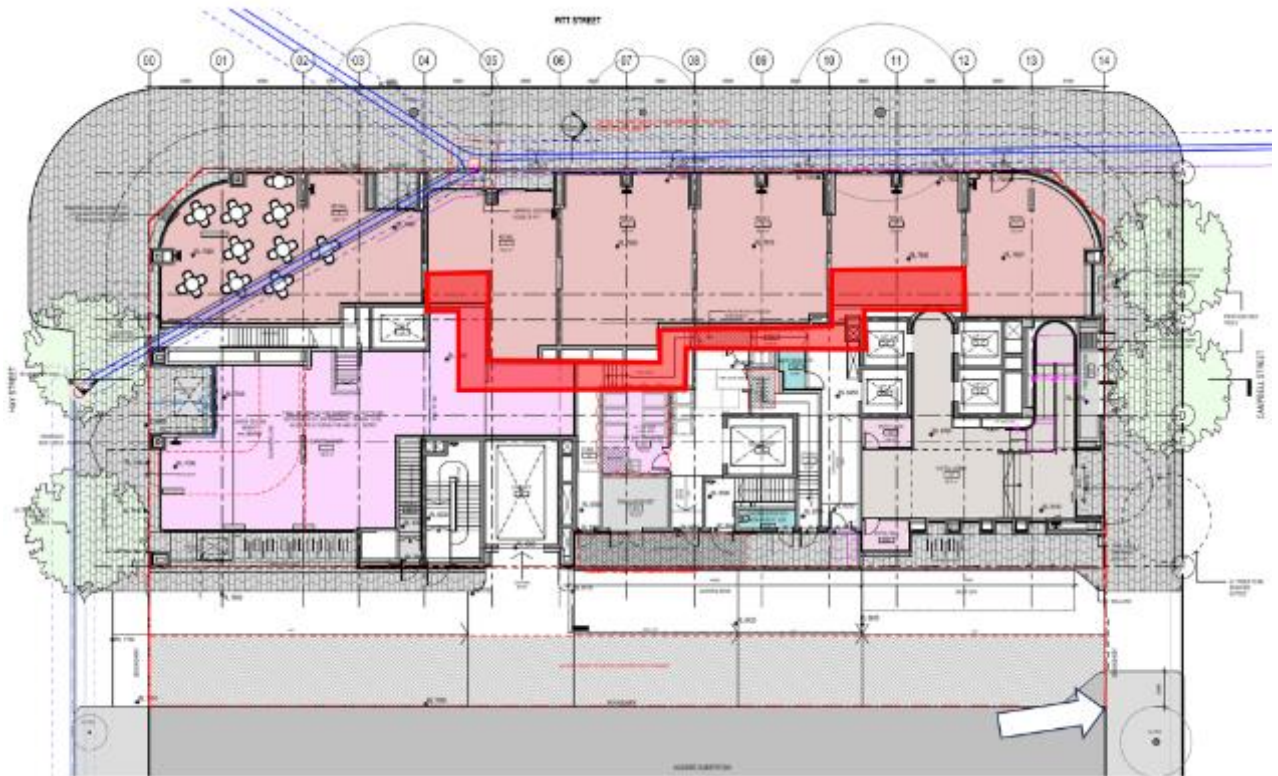
Figure 35: Proposed ground floor plan showing the potential extension of the service corridor to provide internal back of house access to all the retail tenancies
